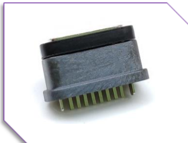
A25WP-F-V-B-08 Waterproof USB Type C 8pin Female Vertical Dip Type
