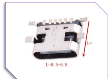
A25-F-M-D-6 USB Type C 6pin Female SMT Type
